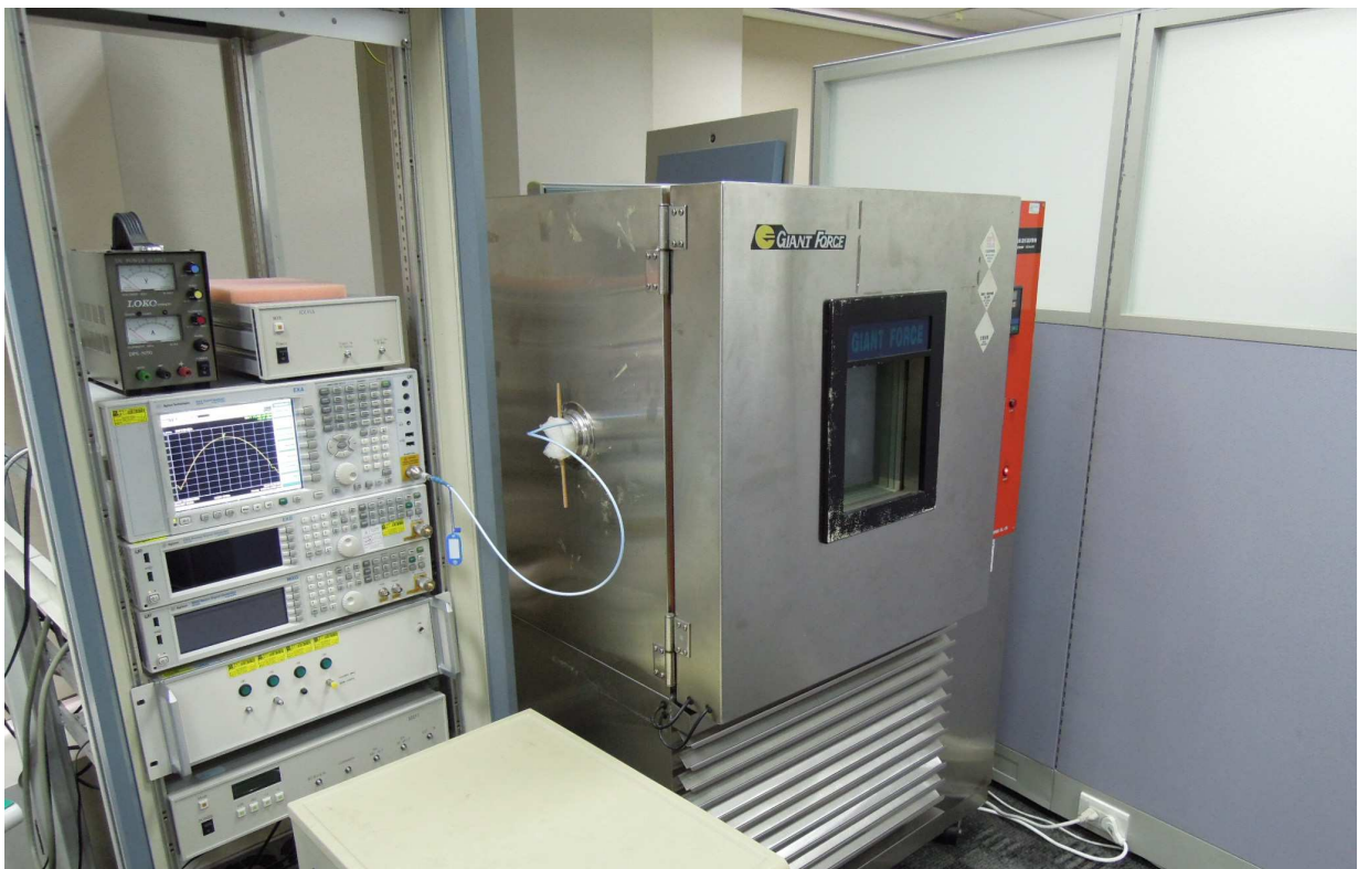
Photograph 4: Set-up for Conducted testing
