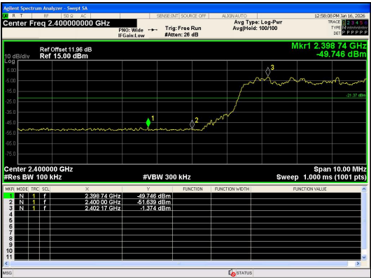
Out Of Band Emission(Right) GFSK_2-DH5_Channel Hopping
