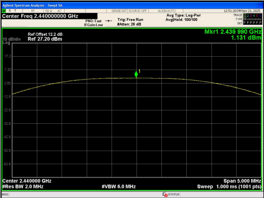
Peak Output Power BLE 2M_Channel 19
