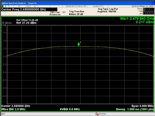
Peak Output Power BLE 2M_Channel 39
