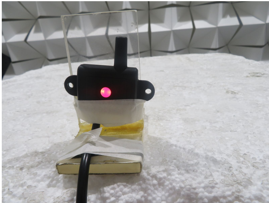
Radiated spurious emission close-up(Above 1GHz)
