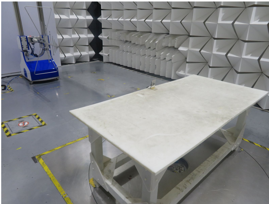
Radiated spurious emission Test Setup-2 (30MHz~1GHz)
