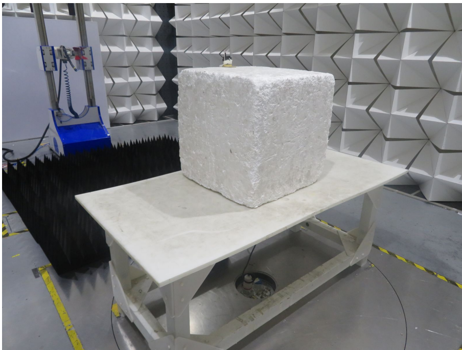
Radiated spurious emission Test Setup-3(Above 1GHz)
