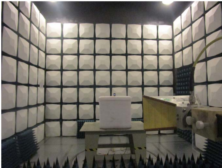
Radiated Emission View (Above 1GHz)
