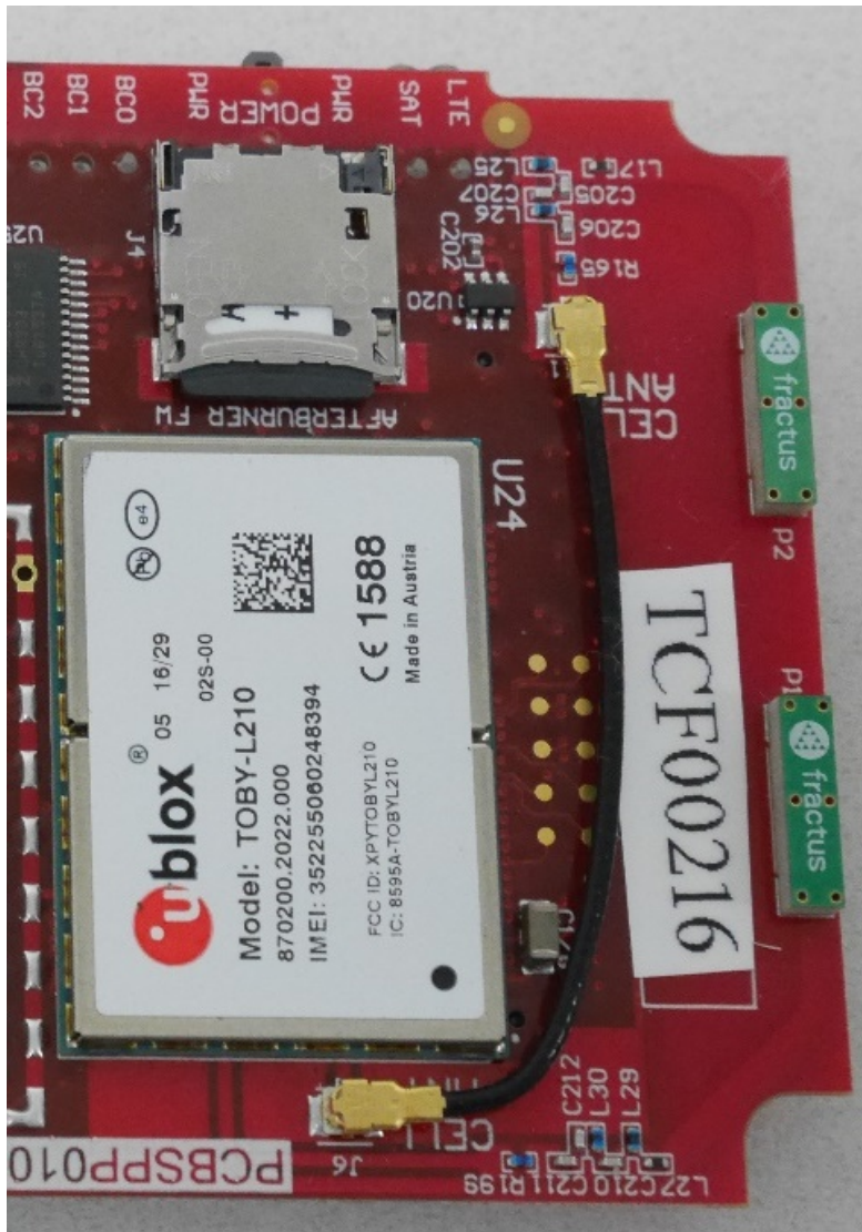
Cellular modem with PCB mount antennas on right
