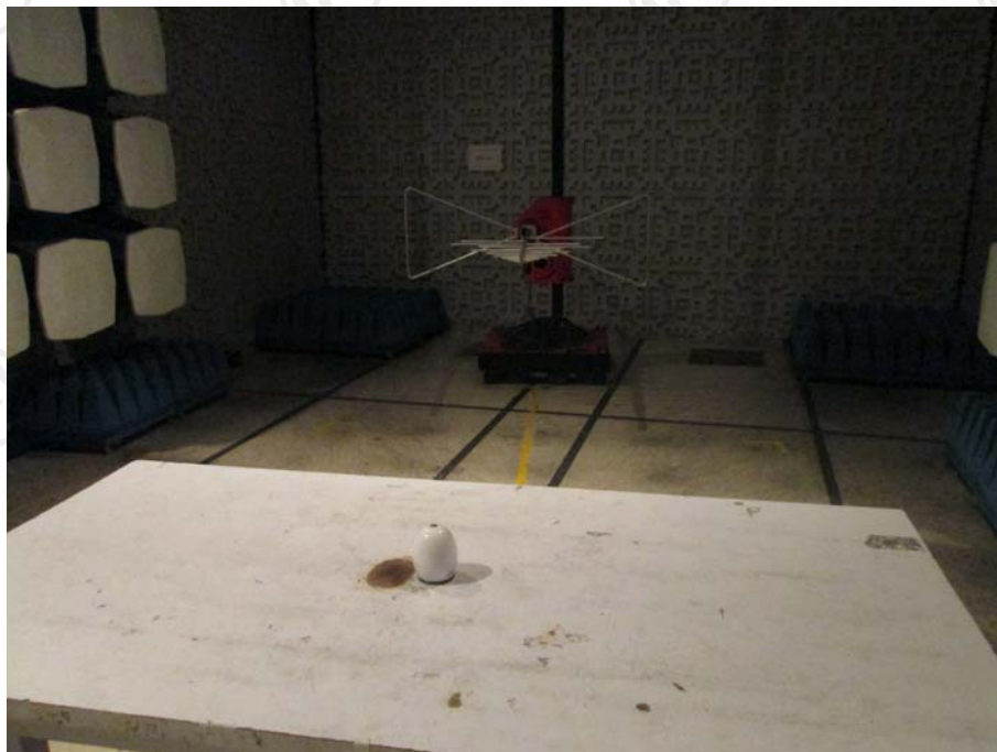
TEST SETUP OF RADIATED EMISSION (30MHz-1GHz)
