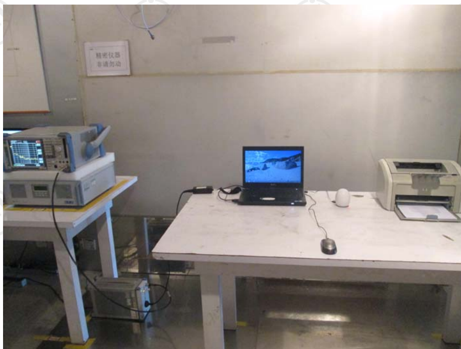
TEST SETUP OF CONDUCTED EMISSION
