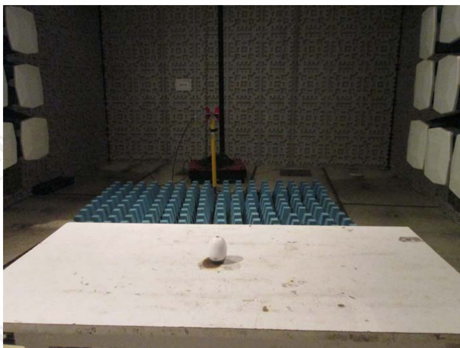
TEST SETUP OF RADIATED EMISSION (above 1GHz)
