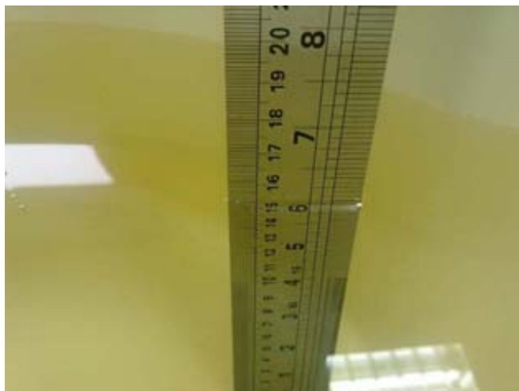
Photograph of the depth in the Head Phantom (835MHz)
