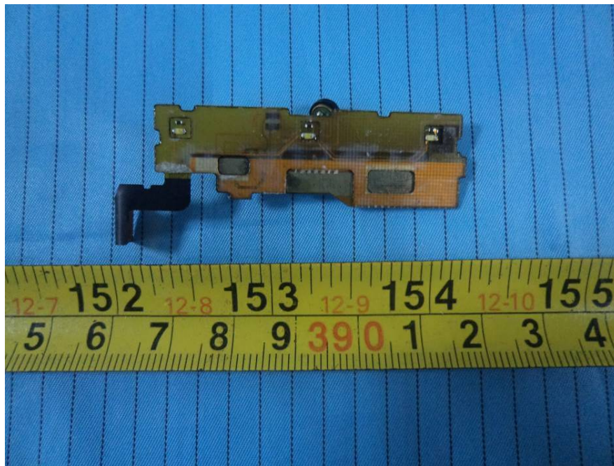
EUT – Sub_Board Bottom View
