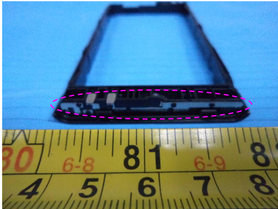
EUT – HSPA&LTE Antenna View
