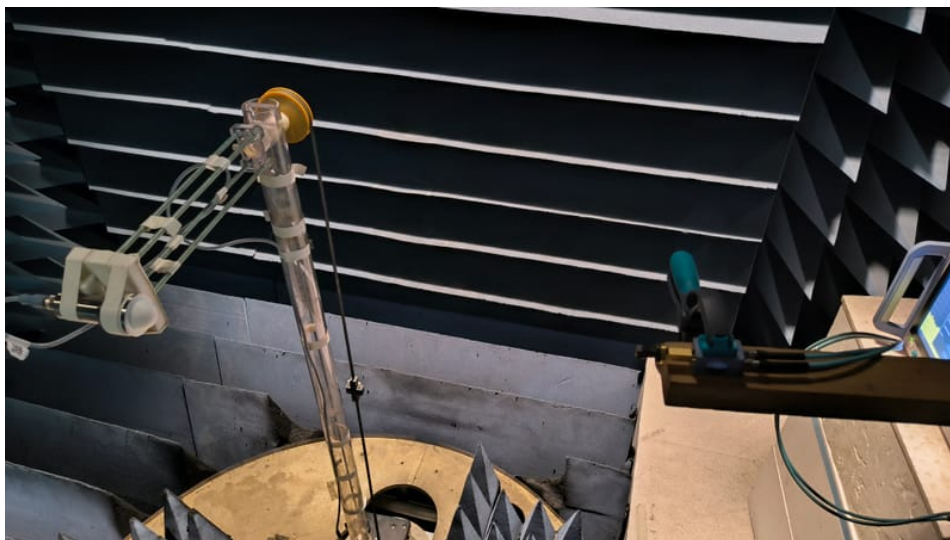
Photo 18: TRP measurement for RSS-295 only
