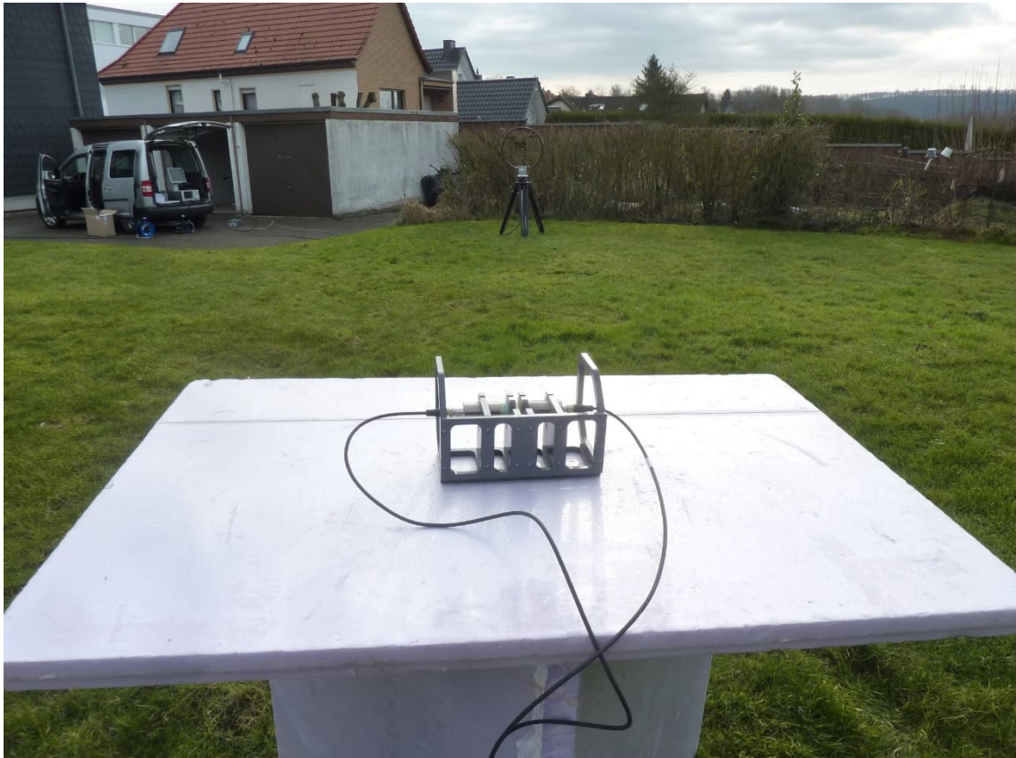
Test setup EUT 1 and EUT2- Radiated emission (Outdoor test side @ 10 m)
