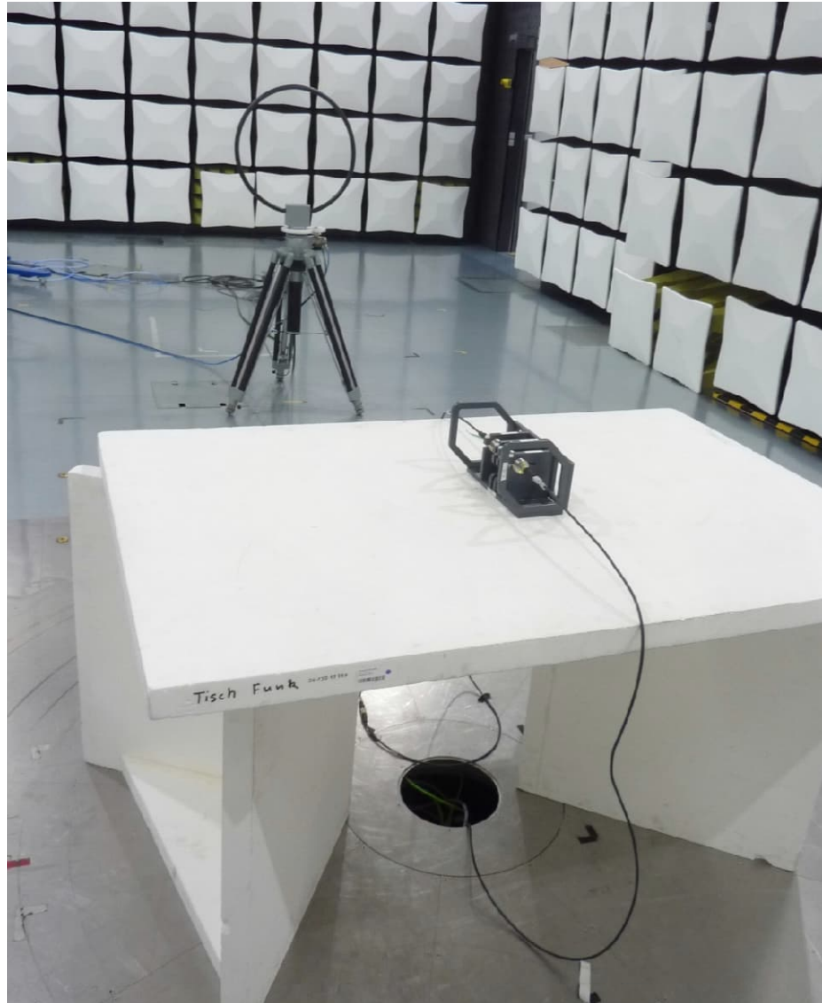
Test setup - Radiated emission (fully anechoic chamber) EUT 1 & EUT 2, 9 kHz – 30 MHz
