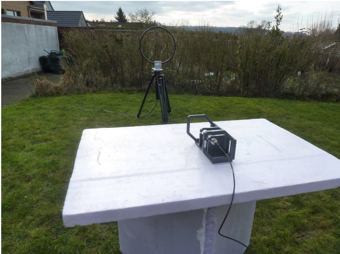
Test setup EUT 1- Radiated emission (Outdoor test side @ 3 m)
