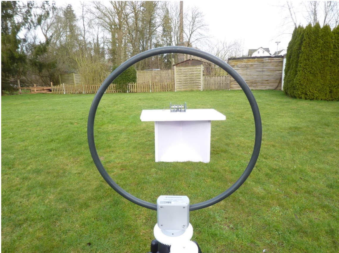
Test setup EUT 1 and EUT2- Radiated emission (Outdoor test side @ 3 m)
