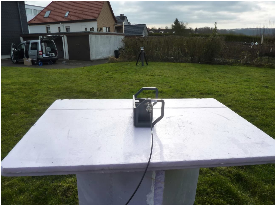
Test setup EUT 1 - Radiated emission (Outdoor test side @ 10 m)
