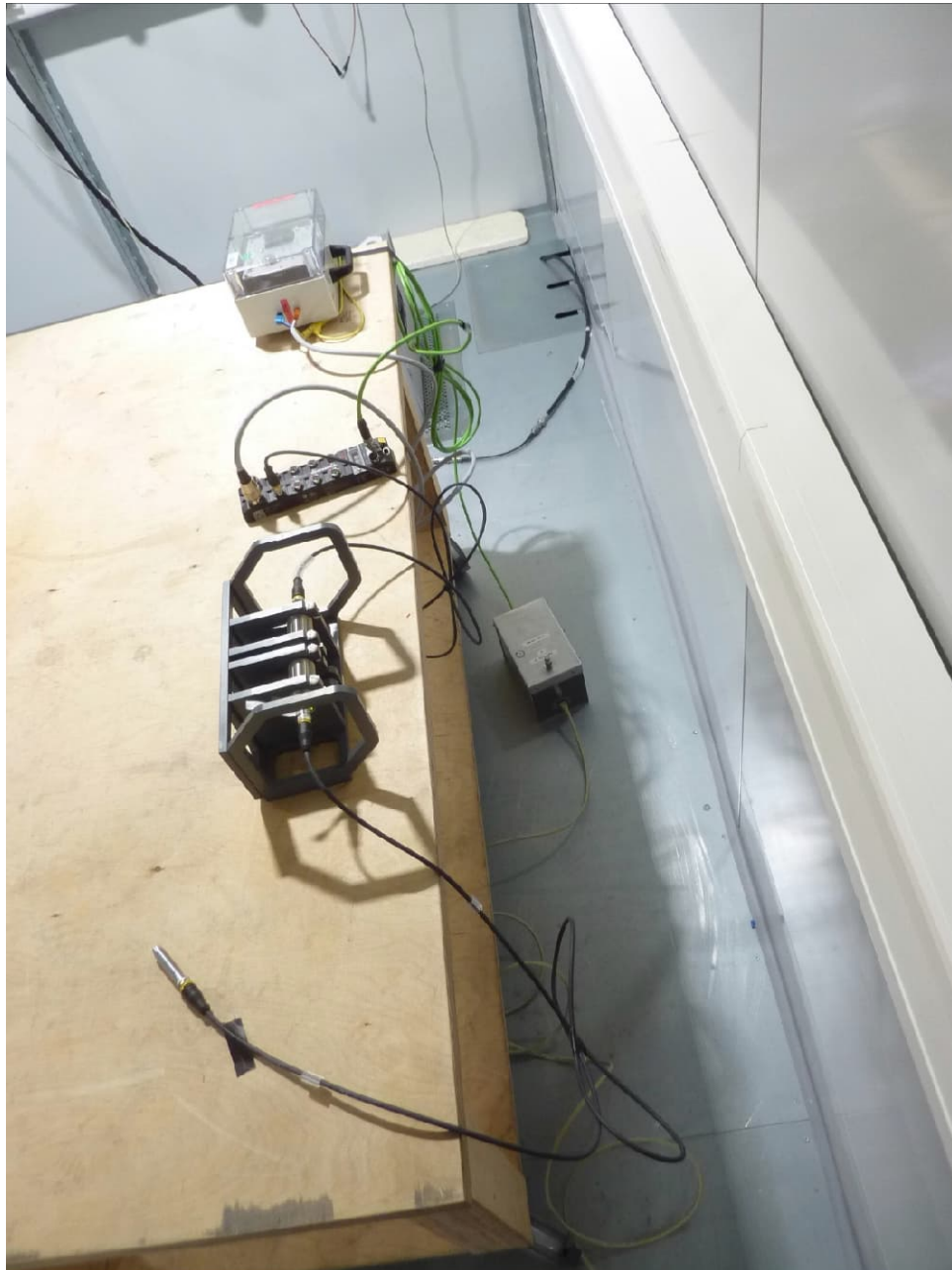
Setup power-line conducted: 150kHz – 30 MHz
