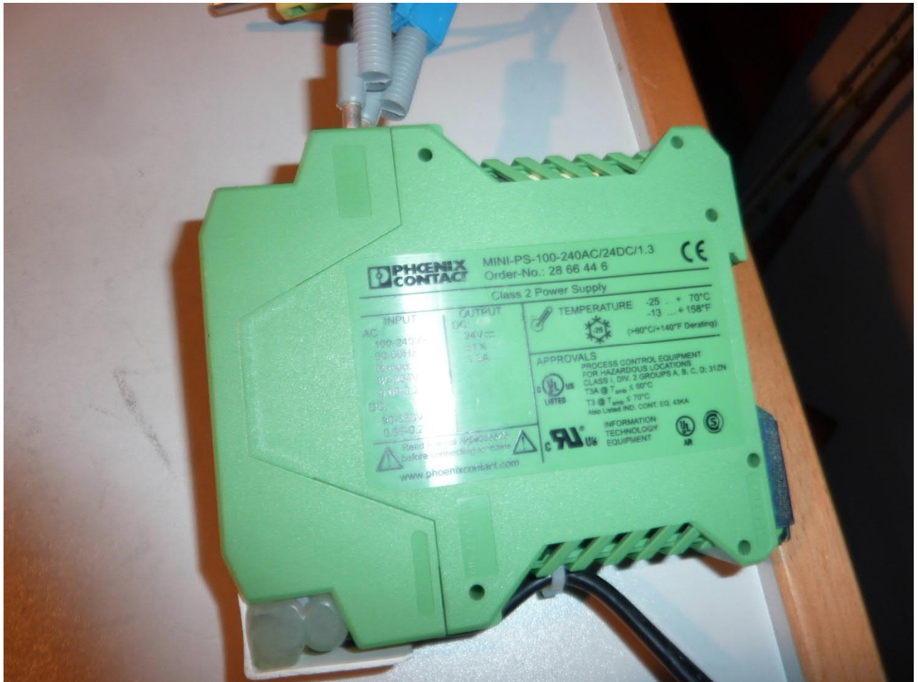
Power adapter MINI-PS-100-240AC/24DC/1.3
