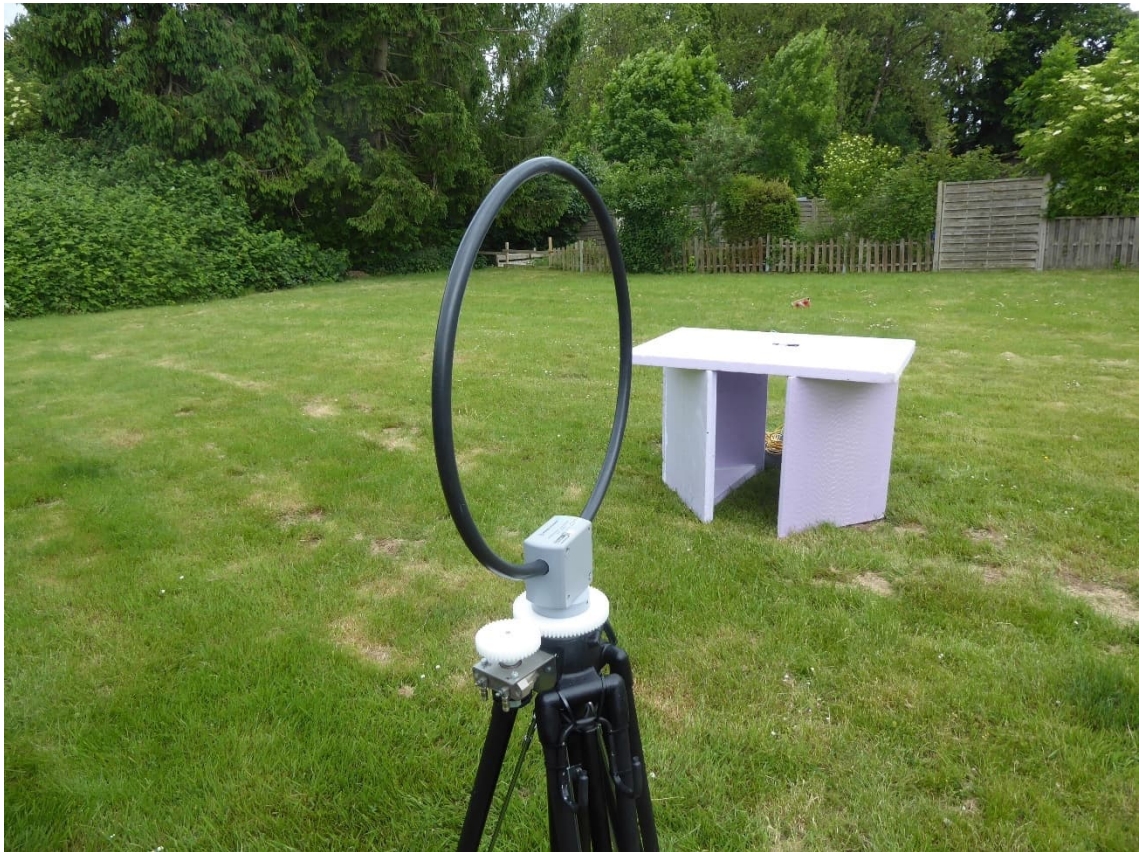
Test setup open area test site (9 kHz to 30 MHz)
