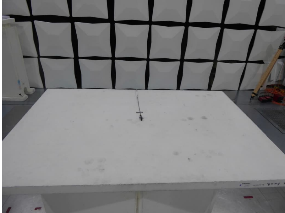
Test setup semi anechoic chamber (Mode 1 – Laying)
