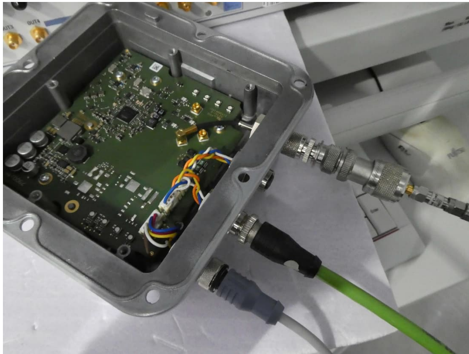
Measurement at internal antenna port
