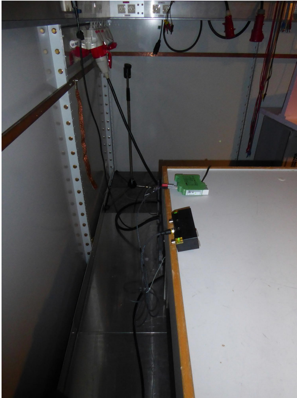
AC Mains conducted emissions test setup
