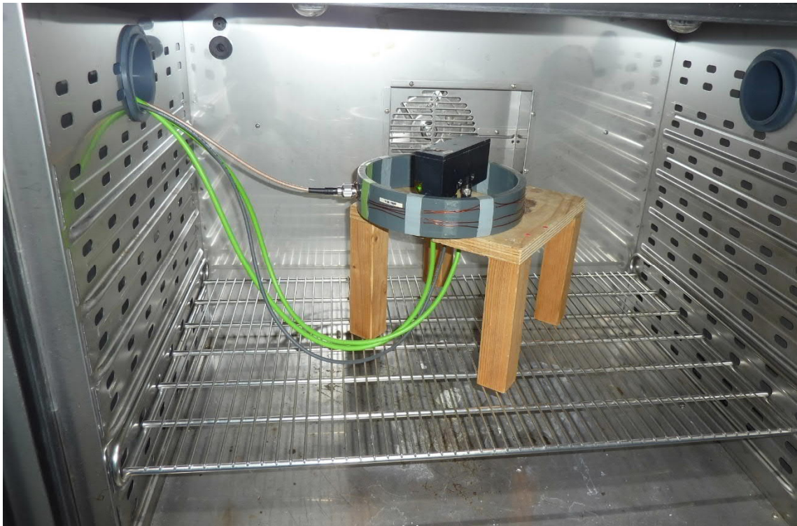
Test setup temperature chamber
