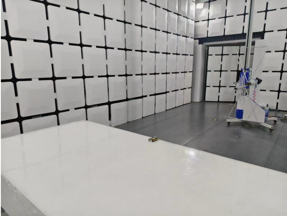
Description: 433M Radiated Emission Test Setup for Below 1GHz
