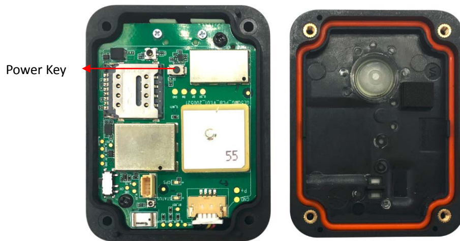
Figure 5. GL50MG Battery Switch and Key
