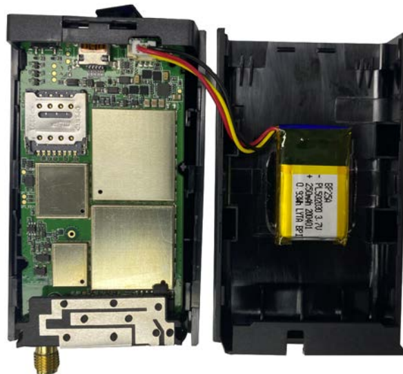
Figure 6. Backup Battery Installation
