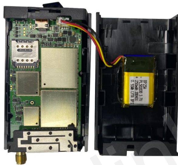
Figure 6. Backup Battery Installation
