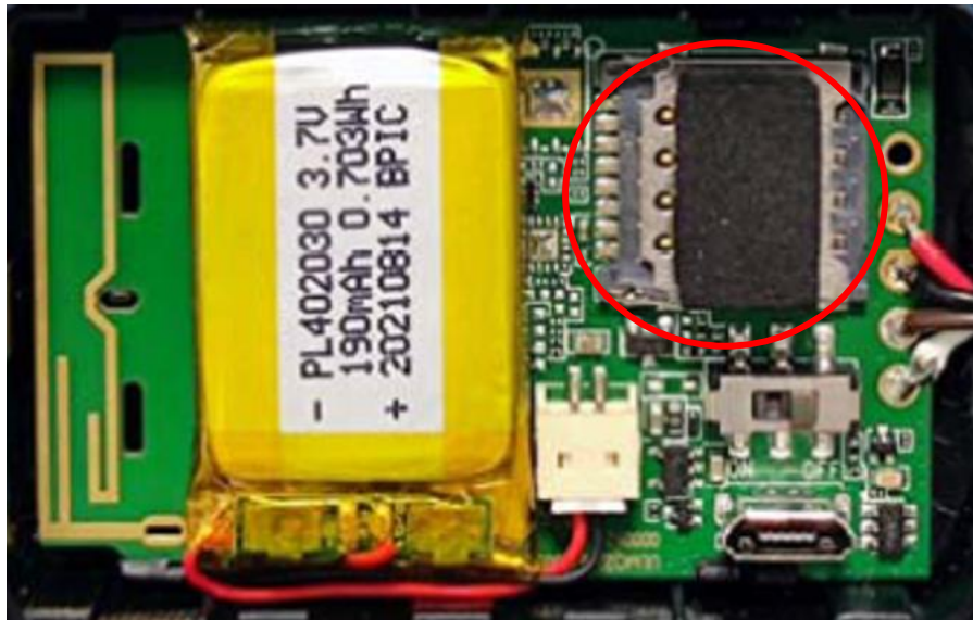
Figure 8. Installing a SIM Card
