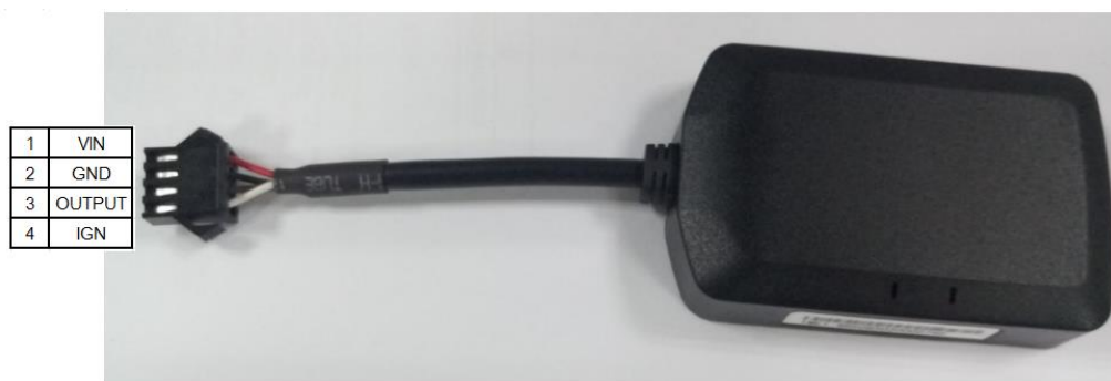
Figure 4. GV50P 4-Pin Cable
