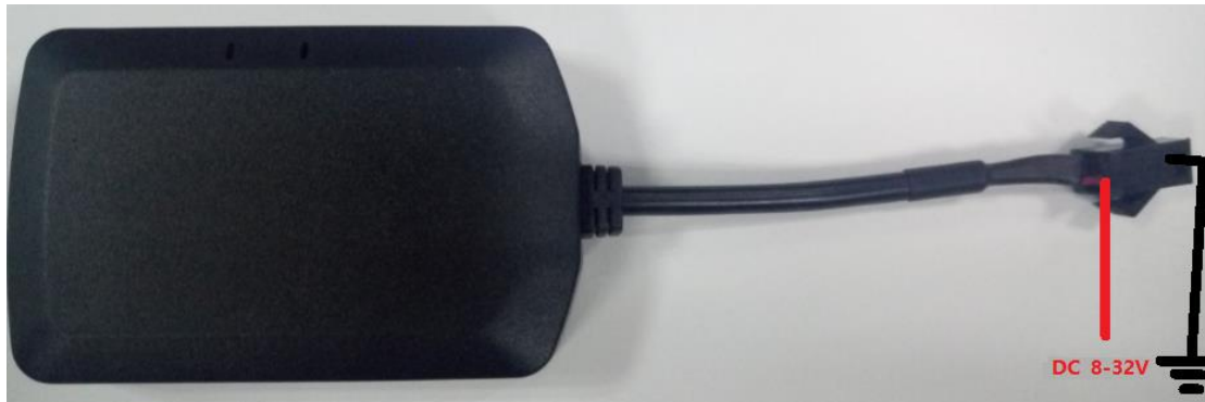
Figure 11. Typical Power Connection
