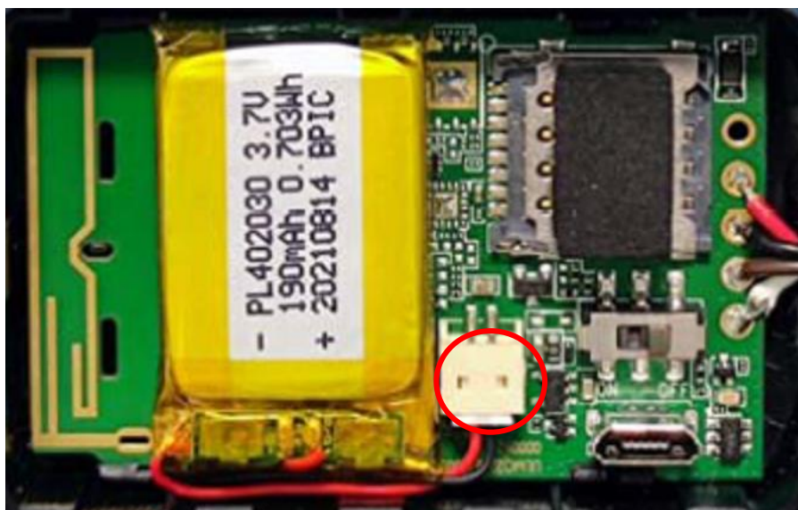
Figure 9. Installing the Internal Backup Battery
