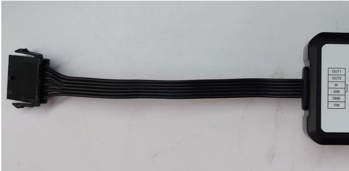
Figure 2.The 6 PIN Connector on the GV55CG
