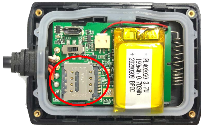
Figure 6. Installing a SIM Card
