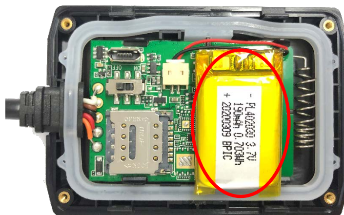
Figure 7. Installing the Internal Backup Battery
