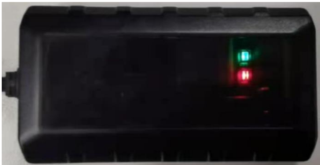
Figure 8. GV57MG V2 LEDs on the Case
