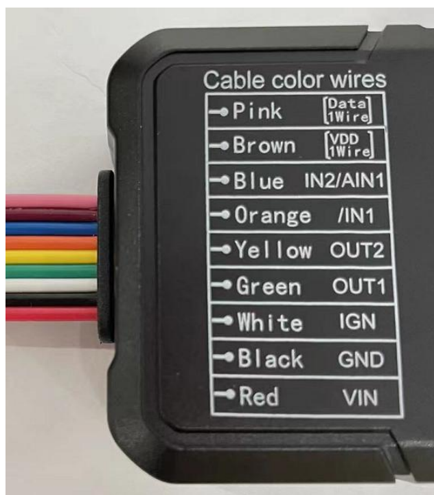
Figure 2: 9-PIN Wire Harness of GV58CEU
