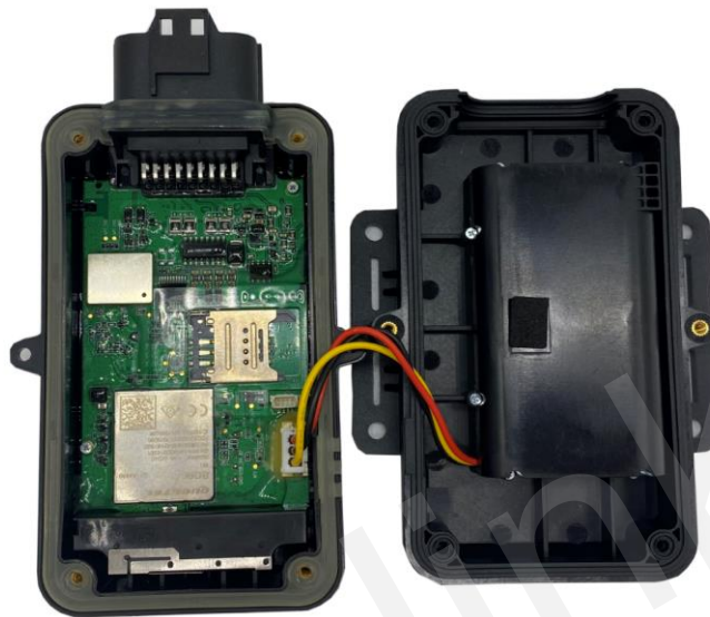
Figure 6. Backup Battery Installation
