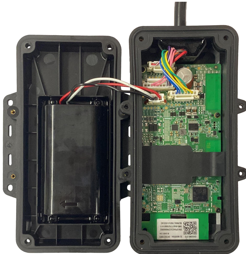
Figure 12. Backup Battery Installation
