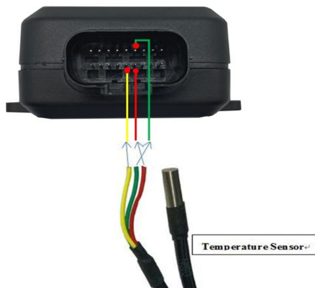
Figure 24. 3 Wires Temperature Sensor 1-Wire Connection
