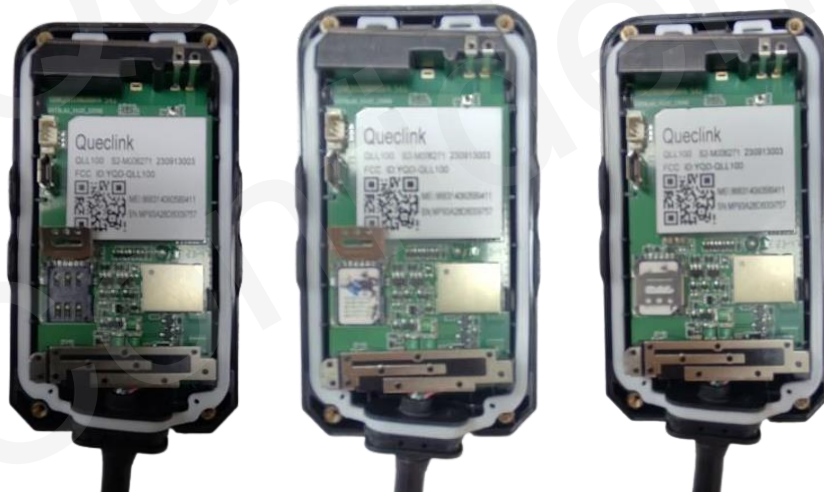
Figure 5: SIM Card Installation
