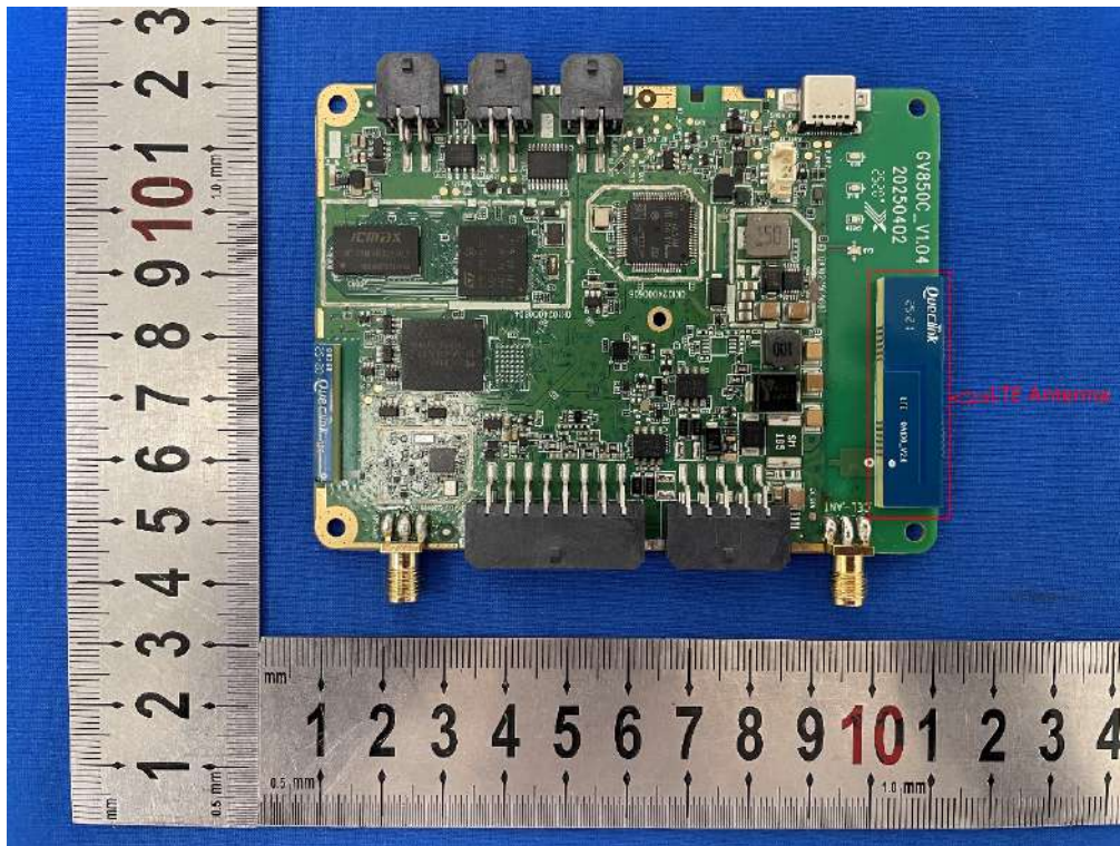
Photo 15: Internal View for LTE Antenna (QA100_V3.0_MIRROR)
