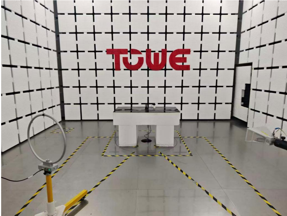
Radiated Spurious Emissions (9kHz to 30MHz)
