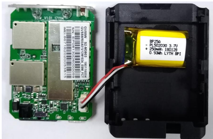
Figure 6. Backup Battery Installation
