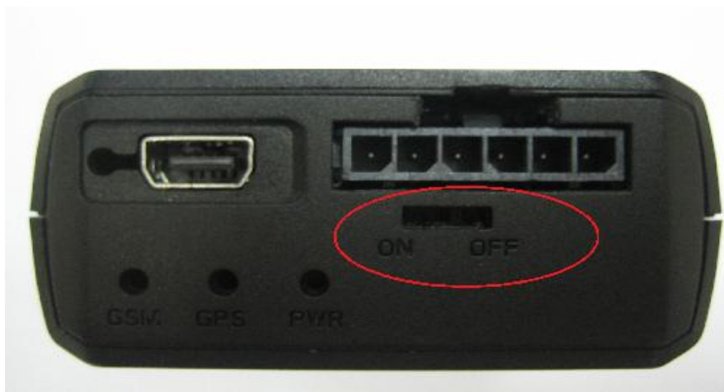
Figure 7. Switch and ON/OFF Position
