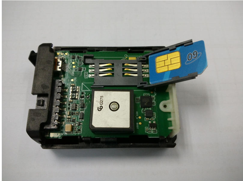
Figure 5. SIM Card Installation
