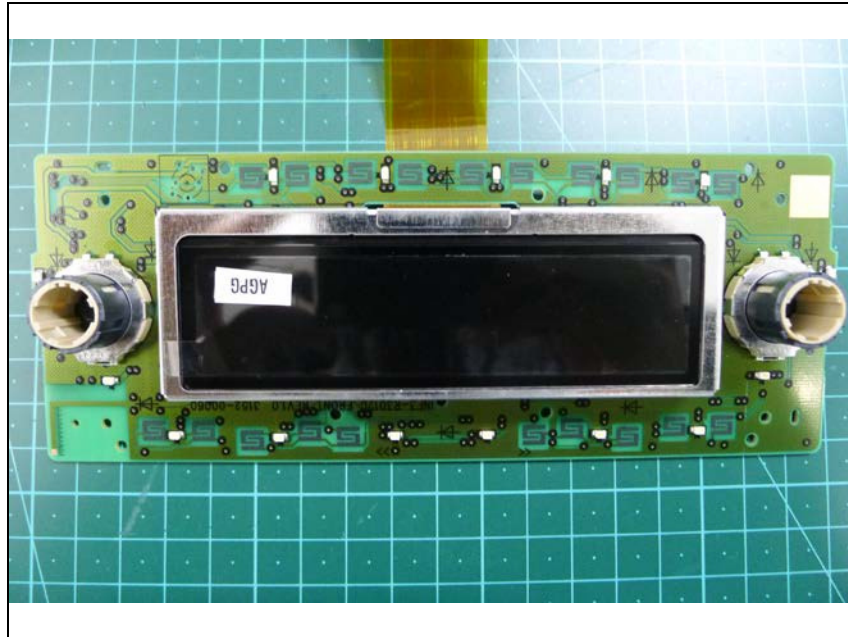
Bottom view of Front PCB
