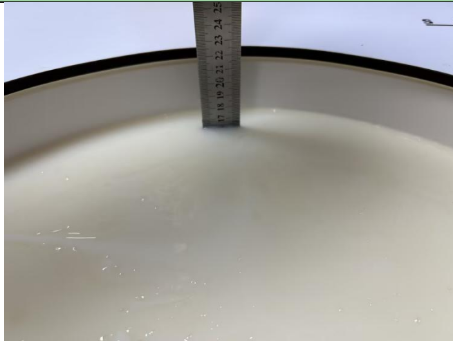
Photo 1: Tissue Simulant Liquid for Head 700-3000MHz
