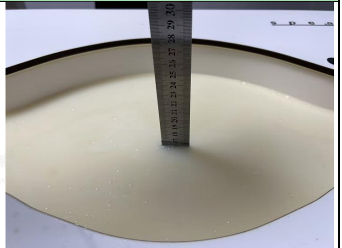
Photo 2: Tissue Simulant Liquid for Head 3000-8000MHz
