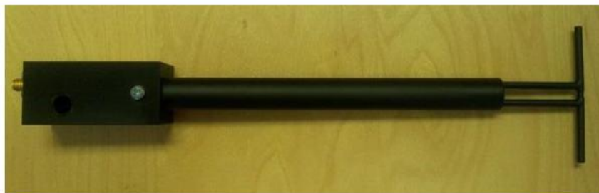
Figure 1 – MVG COMOSAR Validation Dipole
