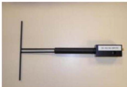
Figure 1 – Satimo COMOSAR Validation Dipole
