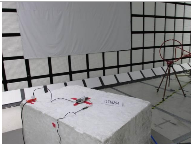
RADIATED BACK PHOTO (BELOW 30 MHz)
