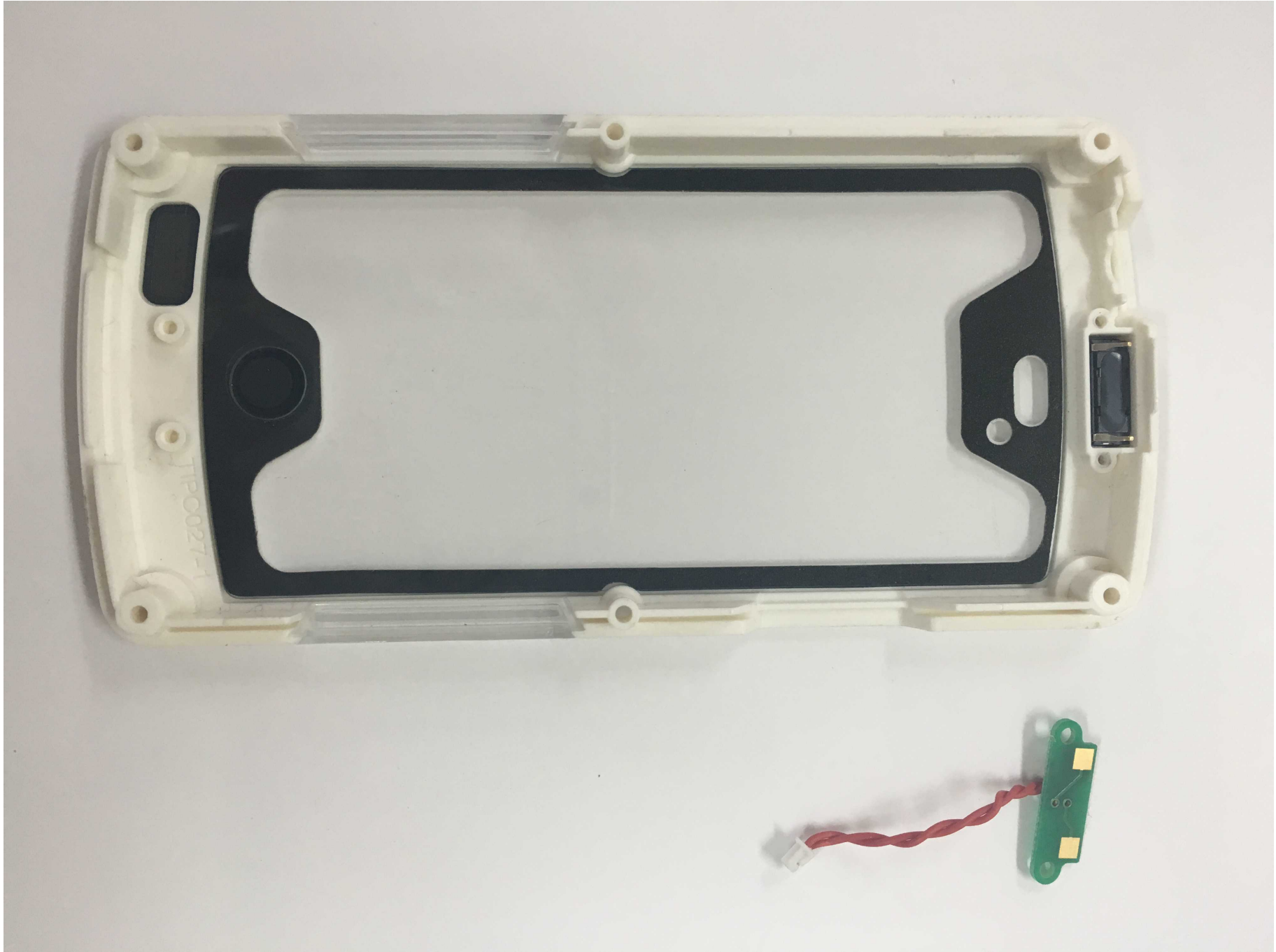
InfineaX - upper enclosure back view and front speaker PCB C018501
