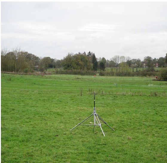
Set up for 300 metre measurements (mag loop end, orange in distance is EUT location)
