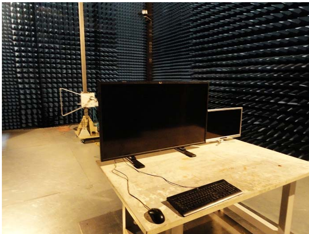
Radiated emission test view-
