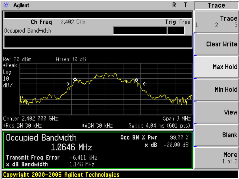
TEST PLOT OF BANDWIDTH FOR LOW CHANNEL
