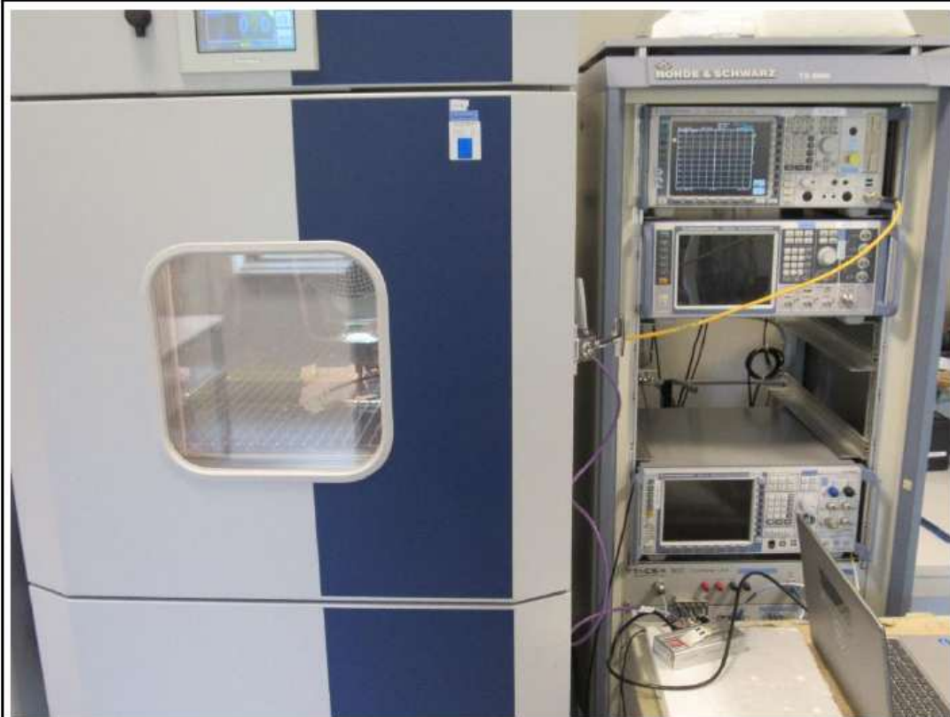
Test setup conducted in climatic chamber view 1
