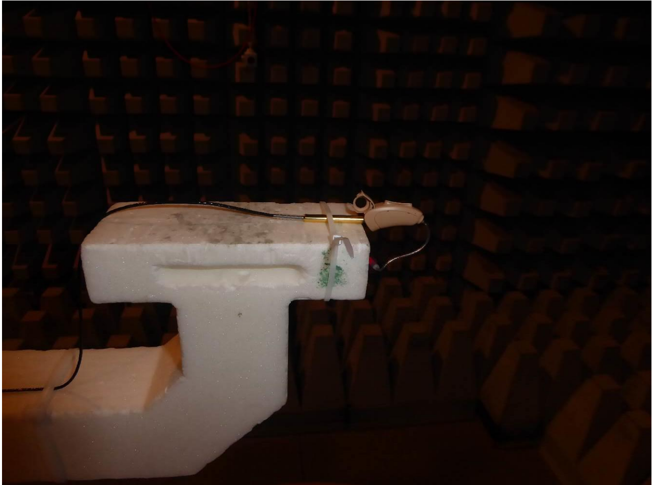
Test setup – radiated test in anechoic chamber
