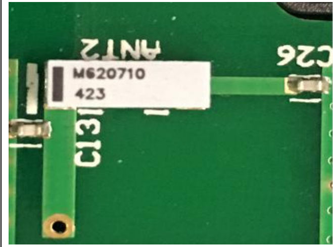
Antenna close View
