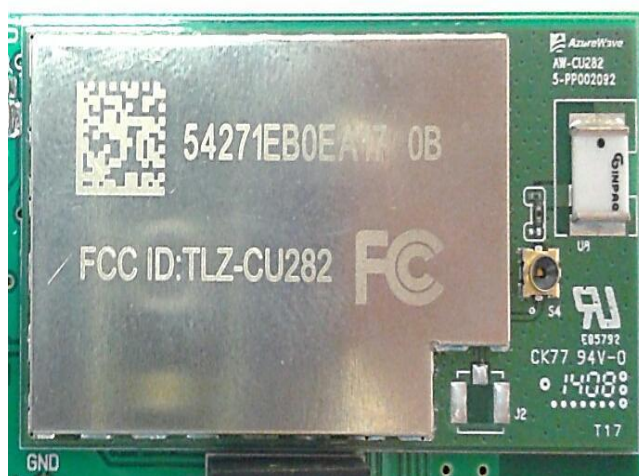
WLAN Module With Shielding
