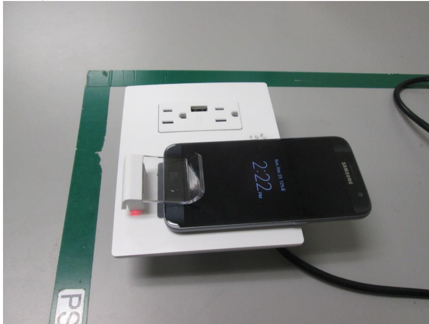
COIL1, RF EXPOSURE SETUP PHOTO
