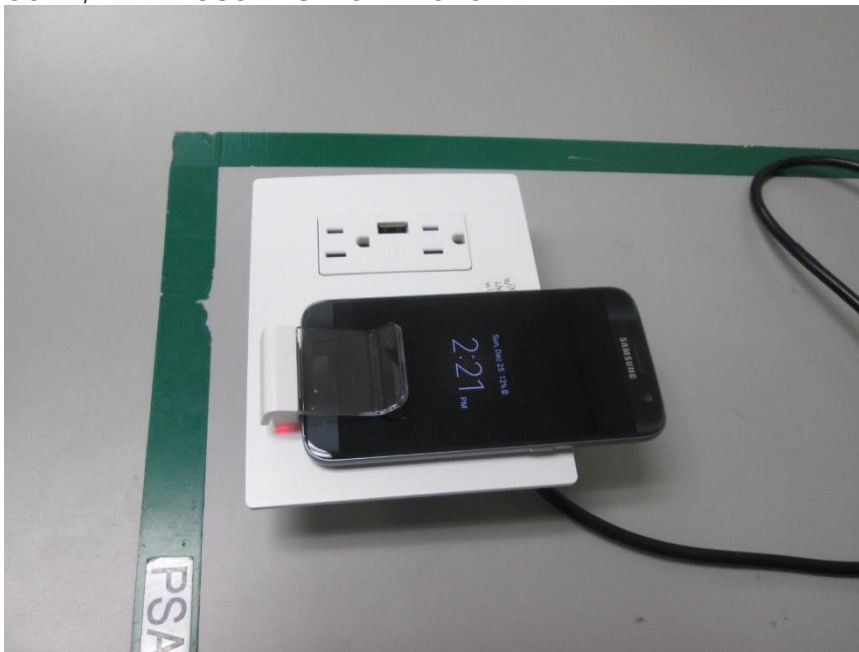
COIL2, RF EXPOSURE SETUP PHOTO
