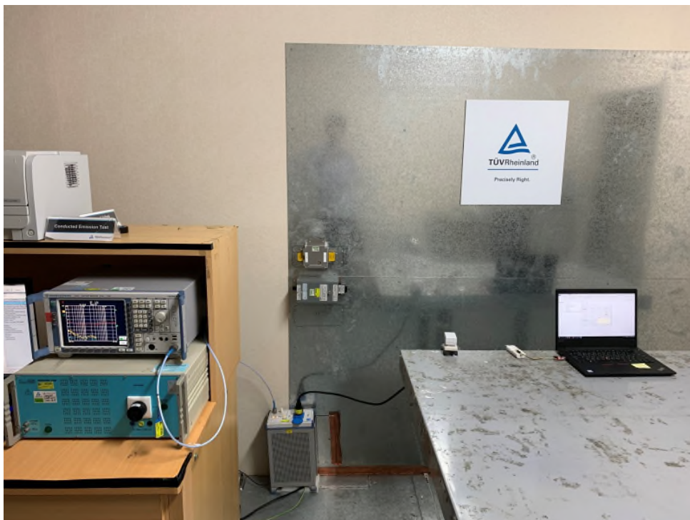
Photograph 8: Set-up for Mains Conducted testing (Front View)
