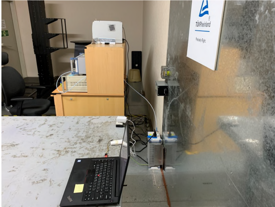
Photograph 7: Set-up for Mains Conducted testing (Back View)
