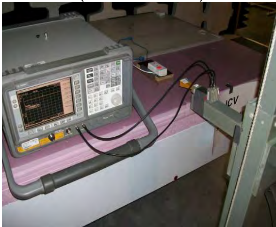
HF Harmonic Mixer (antenna/pre-amp/cables) (18 GHz to 26.5 GHz)
