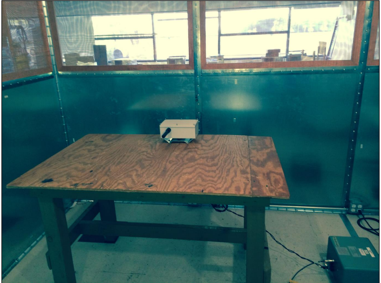
Photograph 5. Conducted Emissions, 15.207(a), Test Setup
