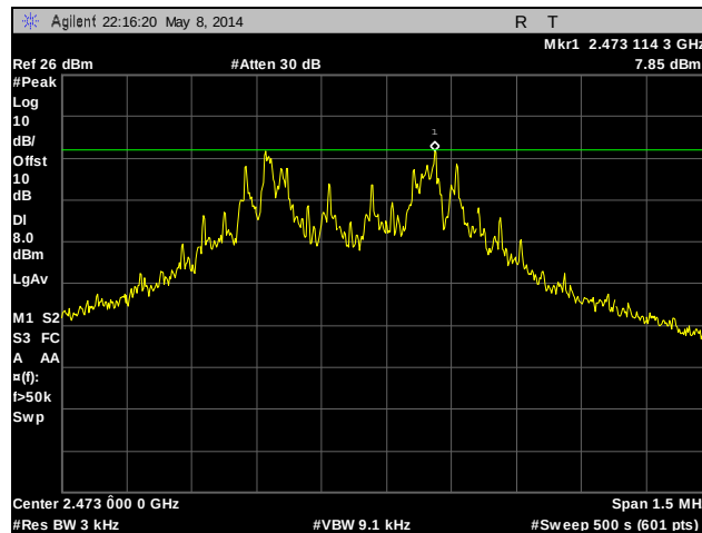
Plot 27. Peak Power Spectral Density, Low Channel
