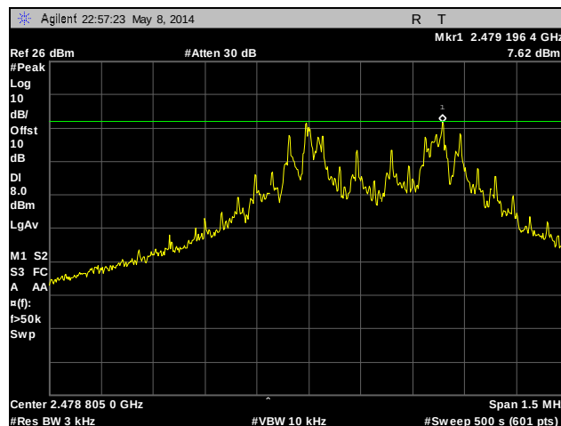
Plot 29. Peak Power Spectral Density, High Channel
