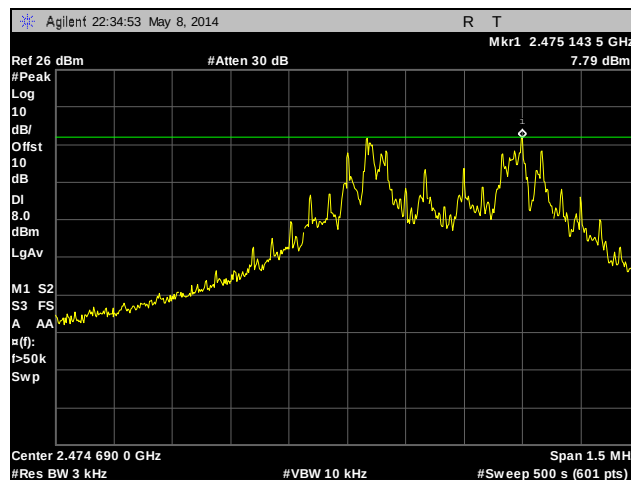
Plot 28. Peak Power Spectral Density, Mid Channel
